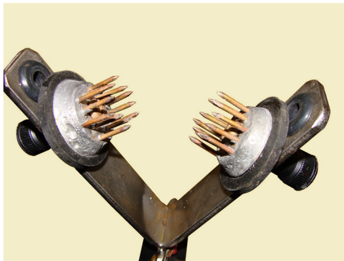
The contact electrodes of a hand-held electrical stunner.
