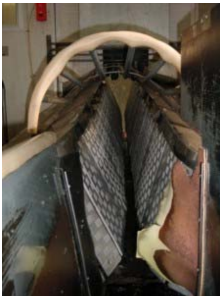
Figure 20 Restrainer conveyor - 'v' formation
