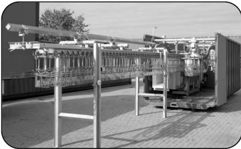
Figure 2: Mobile electrical waterbath stun/kill system
