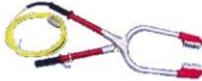
Figure 5 Scissor-type stunning tongs
